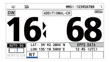
When the receiver detects a carrier and the squelch opens, the following occurs.
